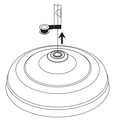
Wrap Teflon tape around the threads of the connecting pipe in a clockwise direction. Thread the shower head on the tape of the pipe and hand tighten as tight as possible.
