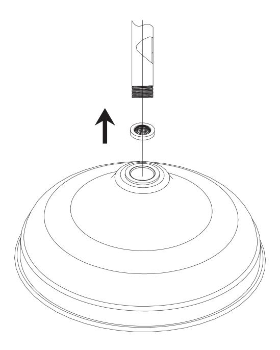
Insert the filter seal into to the shower head.
