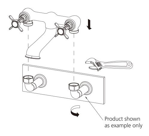
1 Install the faucet onto either the return bends or the cranked legs as chosen. Screw the nut tightly to seal securely.
