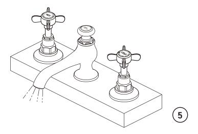
After installing faucet, open the hot and cold supplies to check for leaks. Turn on faucet handle for one minute to flush debris from faucet. Turn off the handle.
