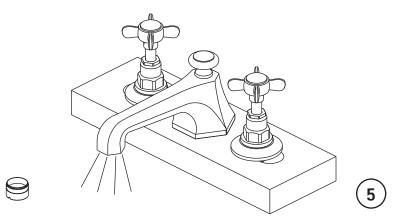
**5** After installing faucet, open the hot and cold supplies to check for leaks. Turn on faucet handle for one minute to flush debris from faucet. Turn off the handle.
