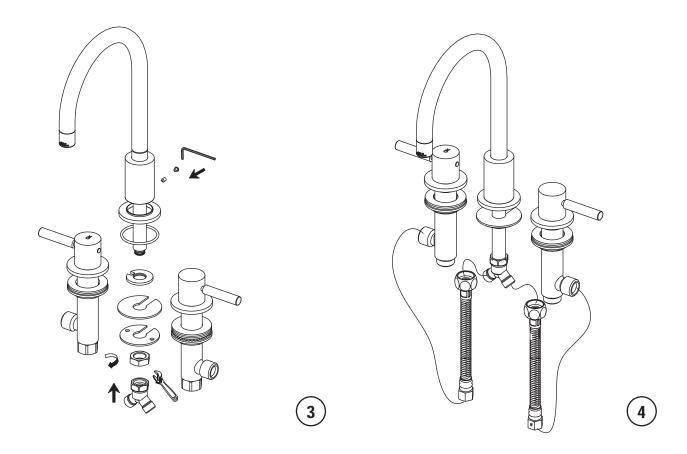
Fit spout and install the connector assembly.
