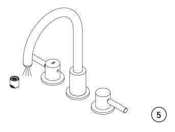
Remove aerator and turn on water to remove any left over debris. Re-assemble aerator.
