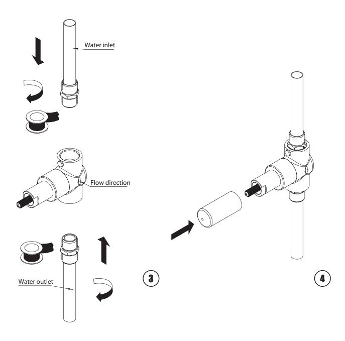
Connect the valve inlet and outlet with water pipes.
