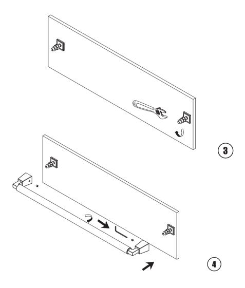
Adjust the direction of the Stud Bolts and tighten the nuts.
