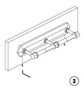
Place assembly over the mounting bracket with set screws facing up. Tighten the set screws.
