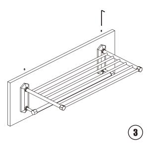
Place assembly over the mounting bracket with set screws facing up. Tighten the set screws.
