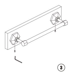
Place assembly over the mounting bracket with set screws facing down. Tighten the set screws.
