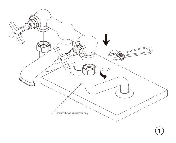
Install the faucet onto either the return bends or the cranked legs as chosen. Screw the nut tightly to seal securely.
