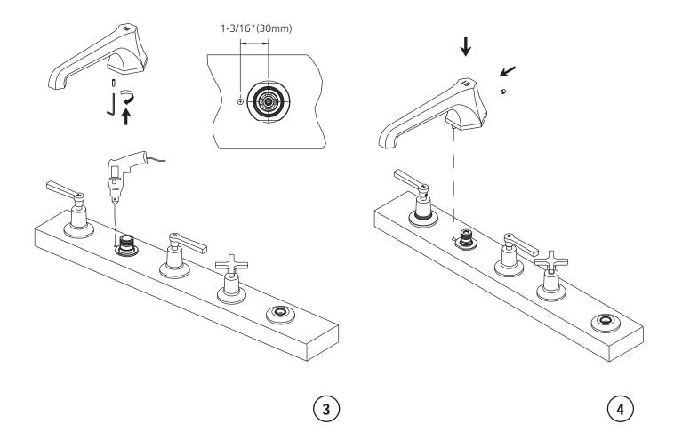
It is recommended that to prevent the spout from accidentally rotating after installation, where possible, the small brass pin should be screwed into the spout base.Drill a 1/4" (5.5mm) diameter hole into the deck to a depth of about 7/16" - 9/16" (11-15mm), following the position indicated in the figure above.
