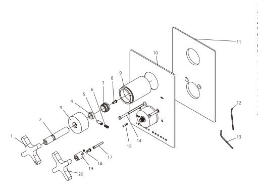
Cross handle (069688-50) Stem extension (110385) Canopy (018958) Clip (012242) Button (036276) Spring (005157) Adaptor (067897) Screw (008154) Sleeve (041724) 9 Back plate (006507-52) 10 11 Oil seal (068329) Allen key (031003) Allen key (031000) Screw (008793) 12 13 14 15 Pin (003153) 16 Canopy (018421-50) 17 Screw (008994) 18 Screw (008772) 19 Stem extension (110405) 20 Cross handle (069688)
