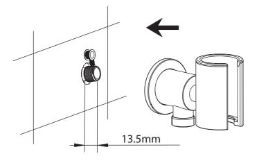
Apply pipe tape on the end threads of the connecting pipe. Please note that the length of the connecting pipe protruded out from the wall surface should be kept as 13.5mm.
