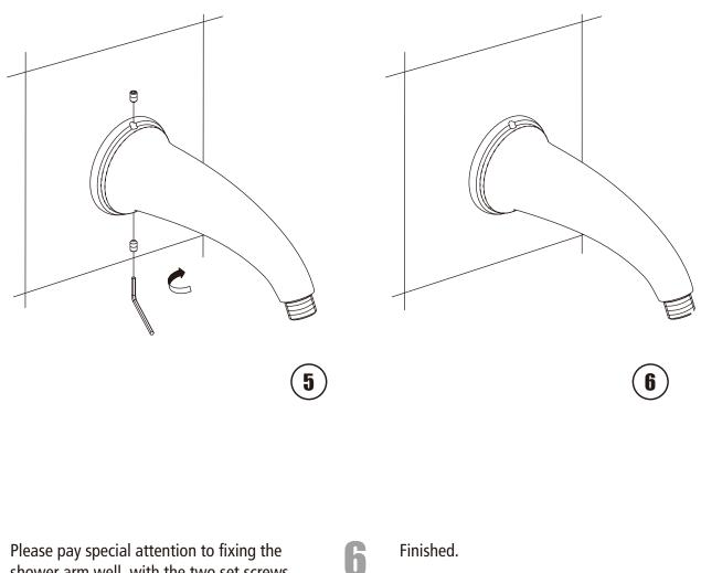
shower arm well, with the two set screws included. The two opposing set screws must be tightened at the same time to prevent the arm leaning to one side".
